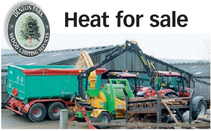
For maximum output Denton Park Estate uses a telehandler to load a table with rollers, ensuring the chipper has a constant supply of timber for maximum output – cut chips can be loaded into trailers or blown into store.
