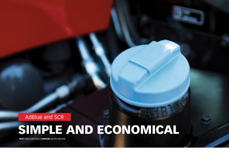
he Selective Catalytic Reduction (SCR) system is used in new low-emissions Tier 3B engines, such as those in the Valtra S Series and new T and N Series tractors, to spray a urea-water solution into the exhaust gases. This reduces nitrogen oxide emissions by up to 80 percent while improving fuel economy by 5 to 10 percent.
