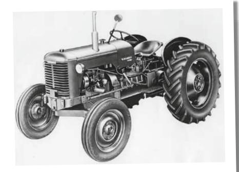
The Valmet 359D was an improved version of the Valmet 33D. The front frame was a single cast component and hydraulic oil was stored separately in a tank by the top of the steps.
