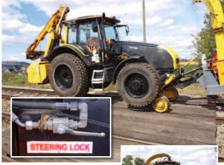
Farm crossings make ideal access points and with rail wheels down and steering locked its ready for off.
