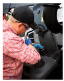
Adding of AdBlue is as easy as refuelling of diesel or adding washing fluid.
