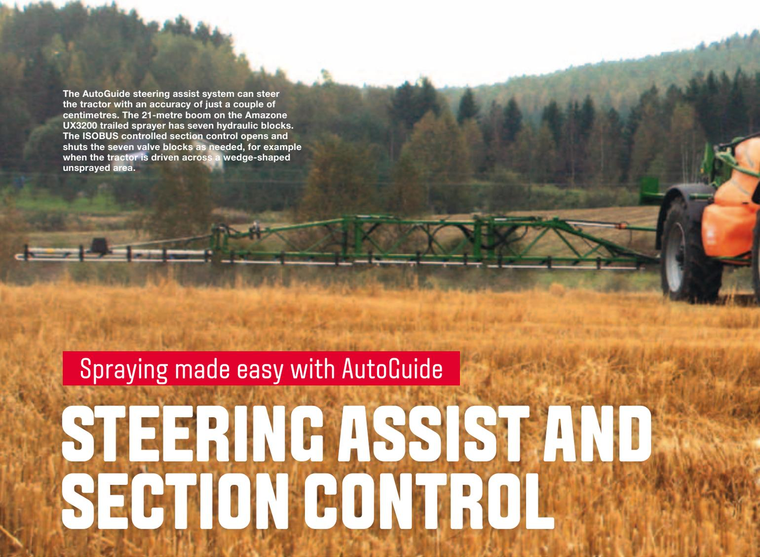
The AutoGuide steering assist system can steer the tractor with an accuracy of just a couple of centimetres. The 21-metre boom on the Amazone UX3200 trailed sprayer has seven hydraulic blocks. The ISOBUS controlled section control opens and shuts the seven valve blocks as needed, for example when the tractor is driven across a wedge-shaped unsprayed area.
