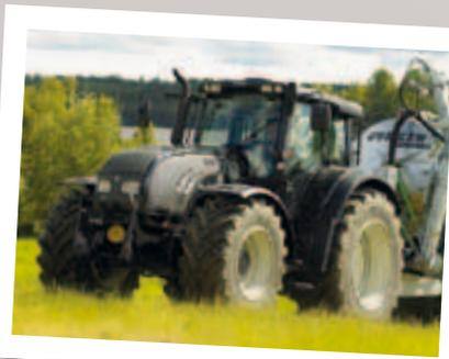
Valtra 202 featured the modern CVT transmission called Direct, which is a combination of mechanical and hydrostatic drive.
