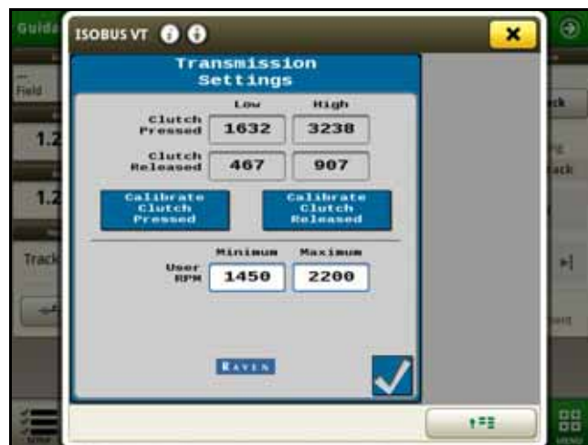
FIGURE 4. Transmission Settings Page for PST Transmissions
